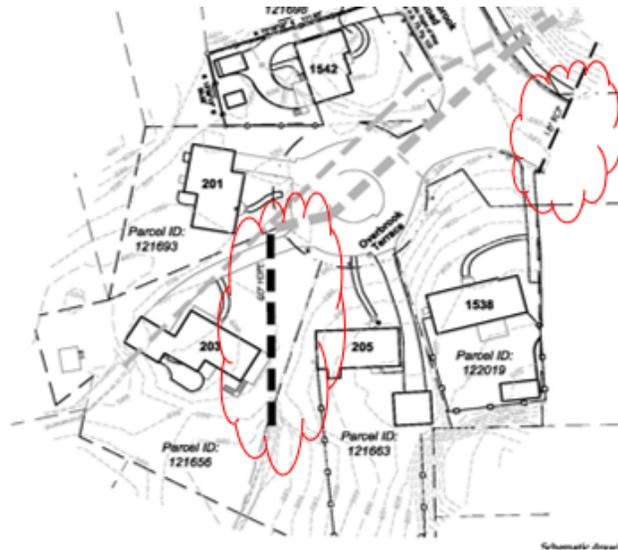
Mr. Patterson reported Alternative 6 would carry higher flow and involves replacing 36" pipe #5 replaced with 60" HDPE, add 60" concrete pipe interceptor alignment and a 18" RCP crossing Overbrook Road. He explained implementing Alternative 6 due to the type of constrictions within the properties involved, it would require the removal of one or both properties located at 201 and 203 Overbrook Terrace to carry the newly installed drain.
